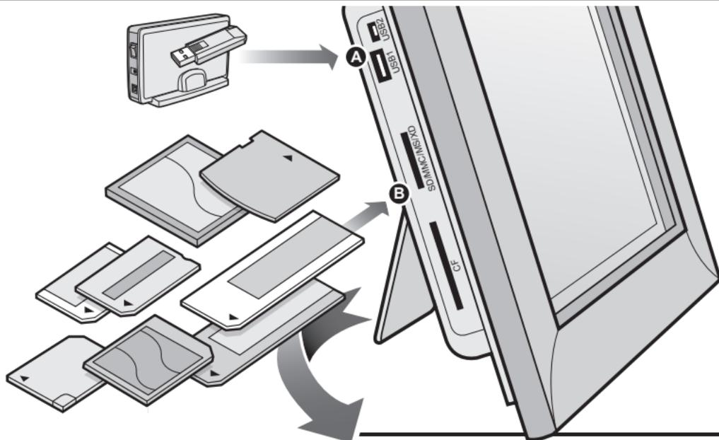
**A** Connect your USB hard drive / thumb drive through the unit's USB port
